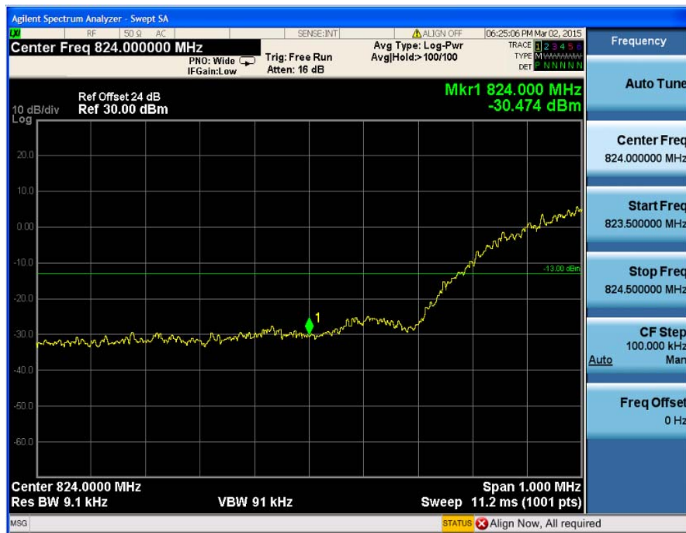
Fig.42 WCDMA Band V-CH4232Band Edge Compliance(HSUPA Subtest5)
