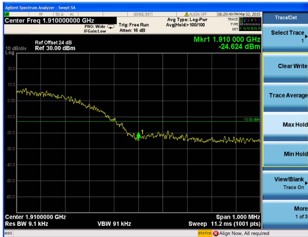
Fig.48 WCDMA Band II-CH9538 Band Edge Compliance(HSUPA Subtest5)
