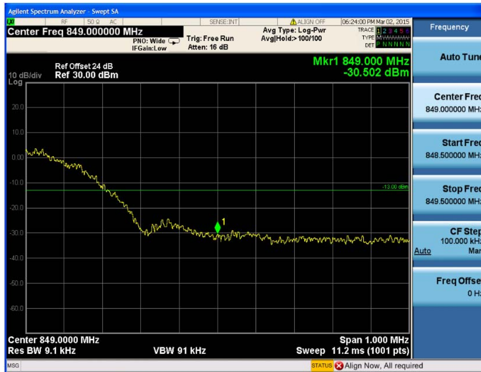
Fig.42 WCDMA Band V-CH4232Band Edge Compliance(HSUPA Subtest5)
