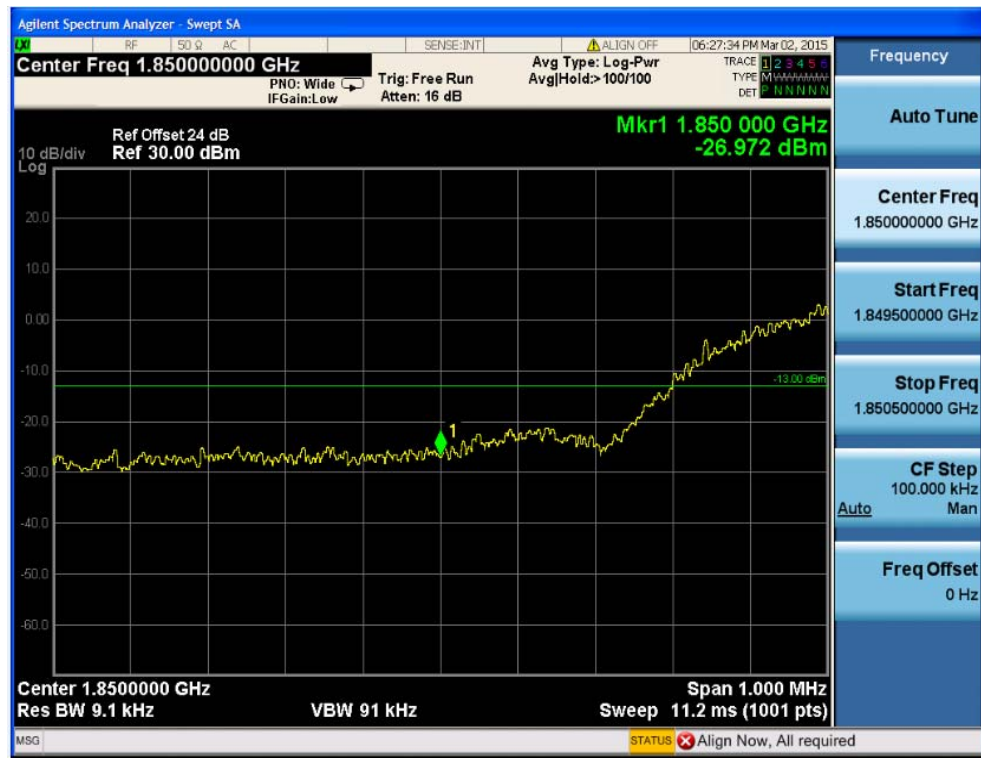
Fig.48 WCDMA Band II-CH9538 Band Edge Compliance(HSUPA Subtest5)
