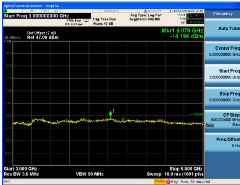
Fig.50 GSM850 on Channel 189 3GHz~9GHz
