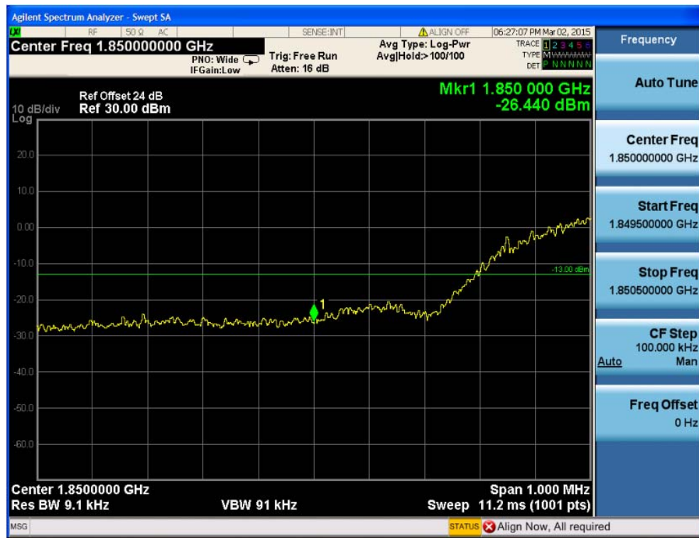
Fig.46 WCDMA Band II-CH9538 Band Edge Compliance(HSDPA Subtest1)
