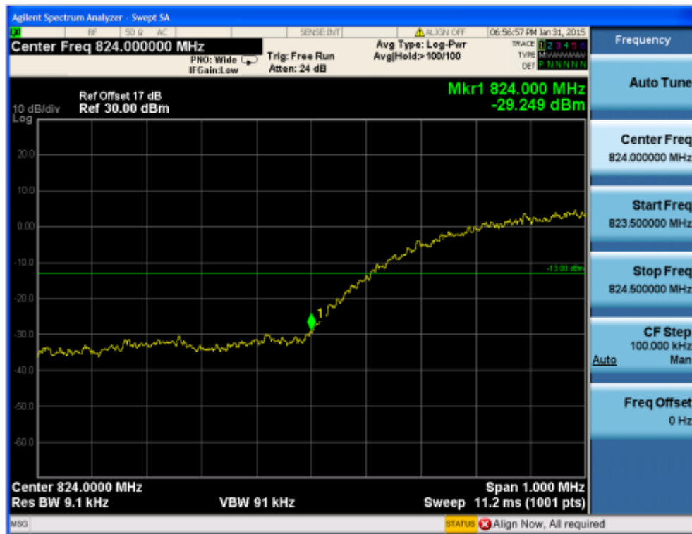
Fig.37 WCDMA Band V-CH4132Band Edge Compliance
