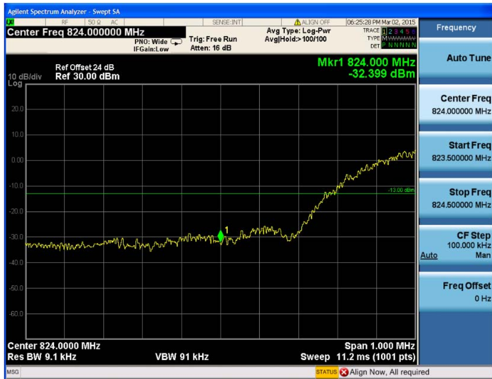
Fig.39 WCDMA Band V-CH4132Band Edge Compliance(HSDPA Subtest1)
