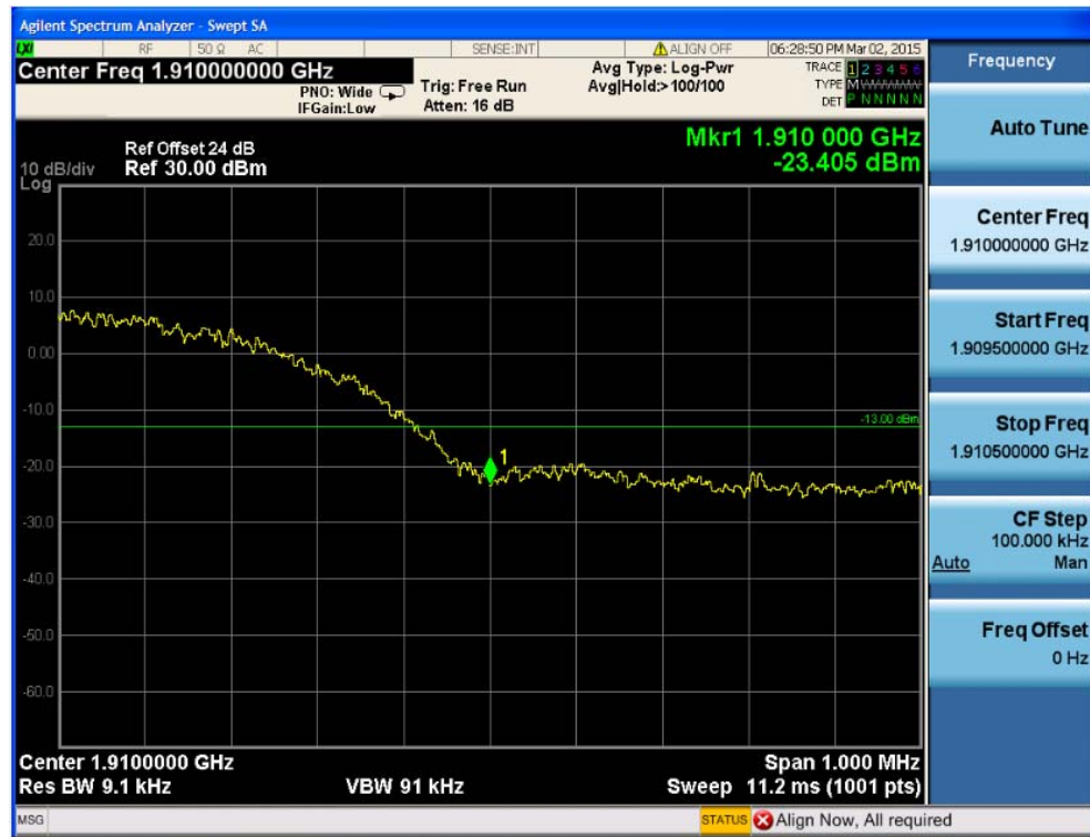
Fig.46 WCDMA Band II-CH9538 Band Edge Compliance(HSDPA Subtest1)
