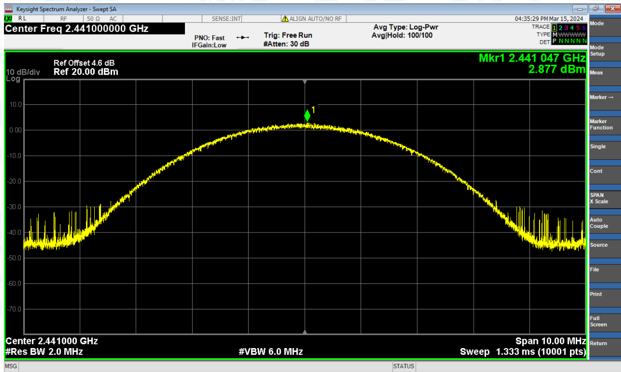
Power NVNT 3-DH1 2441MHz Ant1
