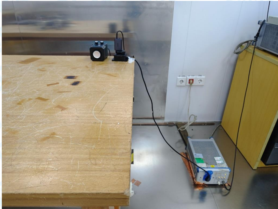
Photo of Setup for Radiated Emission (30MHz~1GHz)
