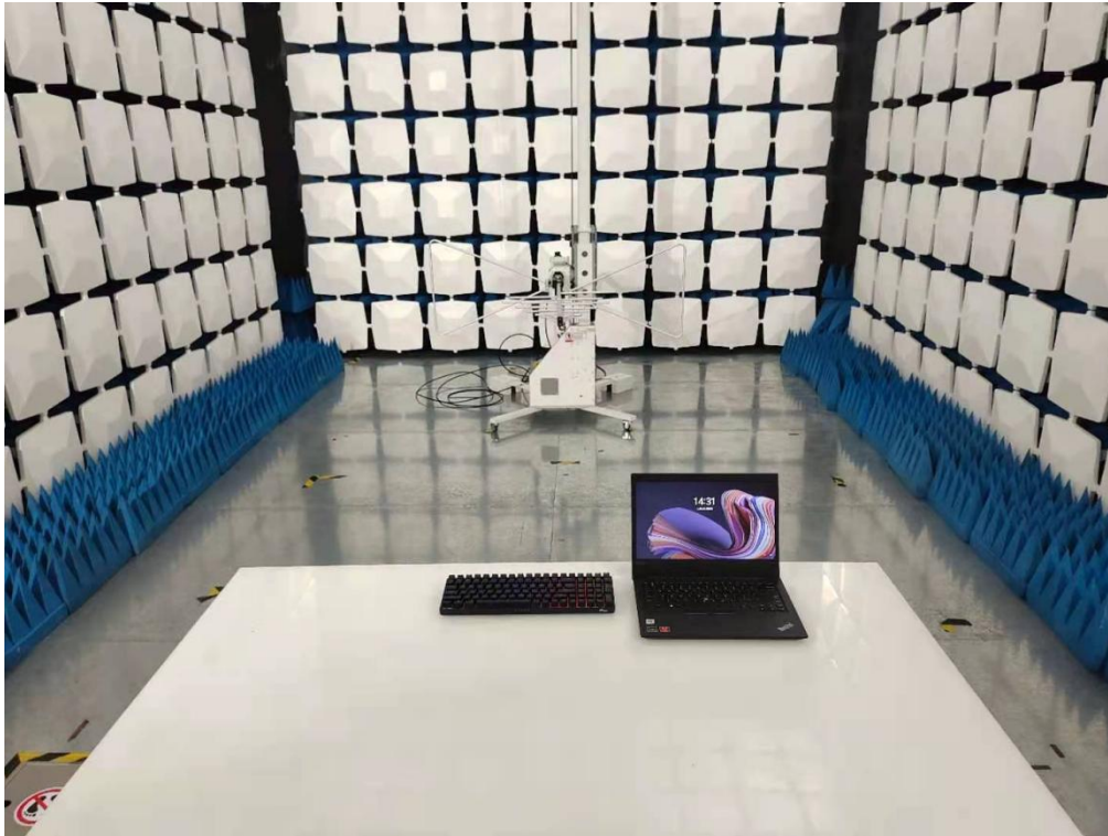
Blow 1GHz for radiated emission test setup
