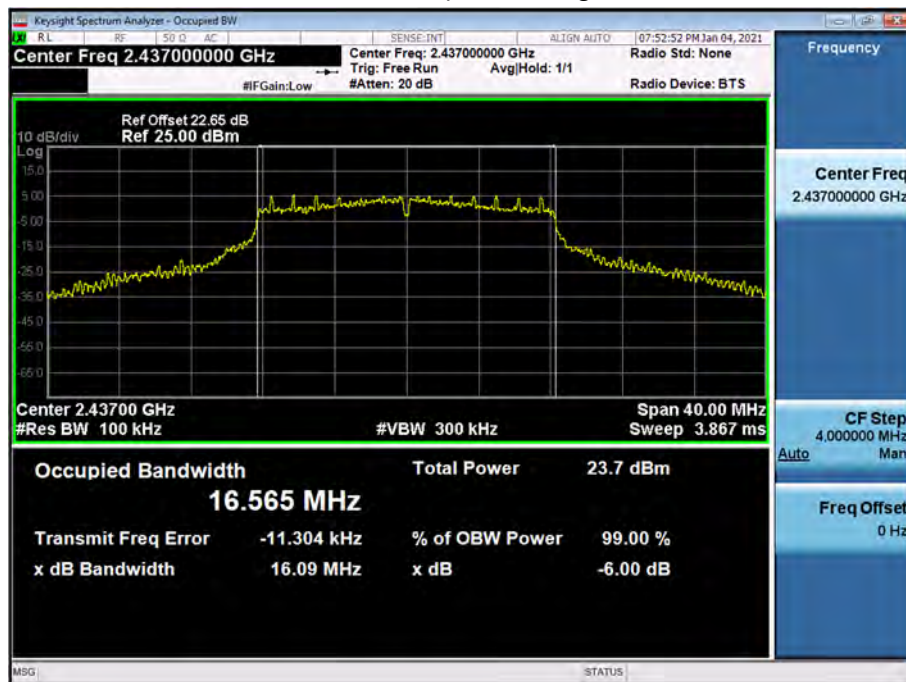
6dB Bandwidth plot (802.11g-CH 6)
