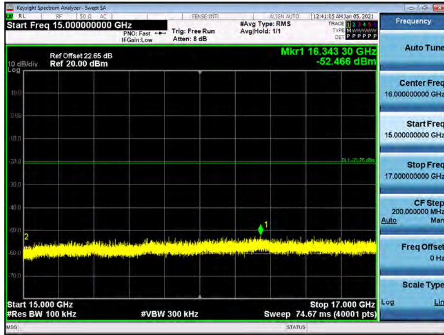
Conducted Spurious Emission (802.11n_Ch.6_MCS 8)
