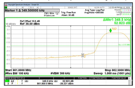
Screen Capture from the spectrum analyzer: Upper Band Edge (125 KHz)
