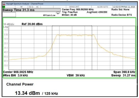
Screen Captures from the spectrum analyzer: 125 KHz High Channel (Hybrid Mode)
