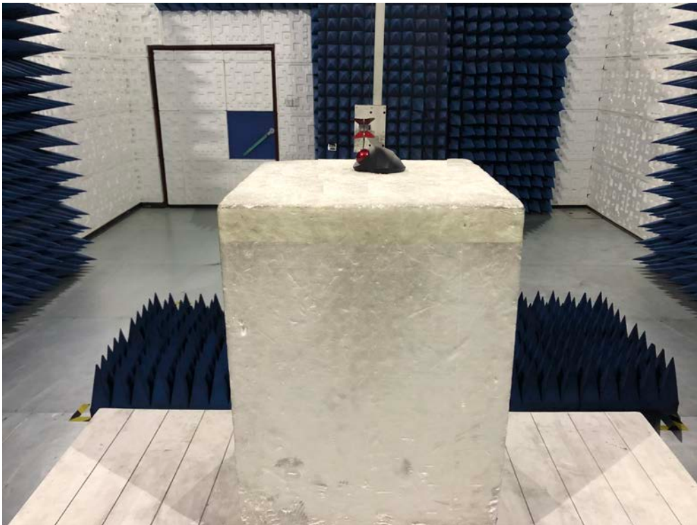
RADIATED EMISSION TEST SETUP ABOVE 1GHZ
