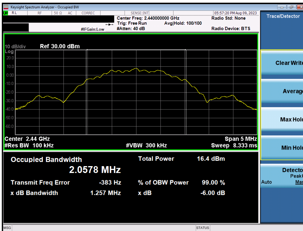
Plot 7-5. 6dB BW & 99% OBW Plot (Bluetooth (LE), 2Mbps – Ch. 19)
