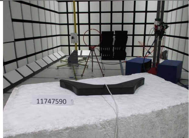
RADIATED BACK PHOTO (BELOW 30MHz)
