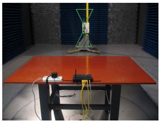
Test Mode: Mode 2: Transmitter by 802.11g Description: Front View of Radiated Test for Above 1GHz
