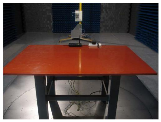
Test Mode: Mode 1: Transmitter by 802.11b Description: Back View of Radiated Test for Above 1GHz
