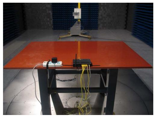
Test Mode: Mode 2: Transmitter by 802.11g Description: Front View of Radiated Test for Under 1GHz
