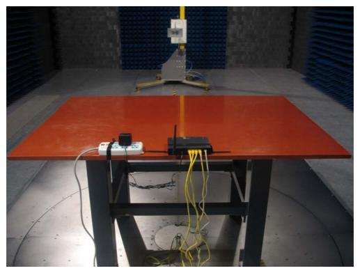
Test Mode: Mode 1: Transmitter by 802.11b Description: Conducted Spurious Emission Test for 18G-25G
