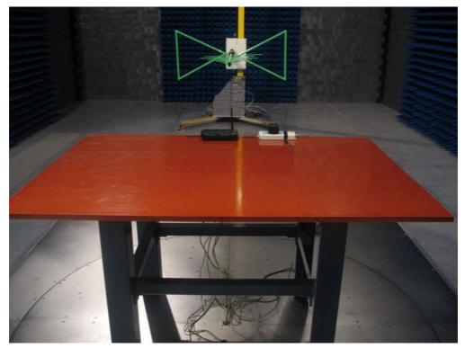
Test Mode: Mode 1: Transmitter by 802.11b Description: Back View of Radiated Test for Under 1GHz
