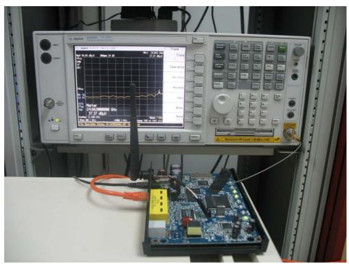
Test Mode: Mode 2: Transmitter by 802.11g Description: Conducted Spurious Emission Test for 18G-25G
