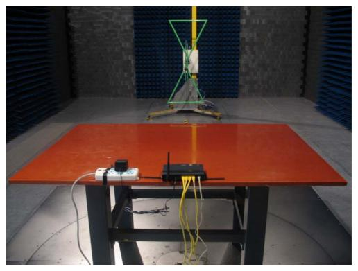
Test Mode: Mode 1: Transmitter by 802.11b Description: Front View of Radiated Test for Above 1GHz
