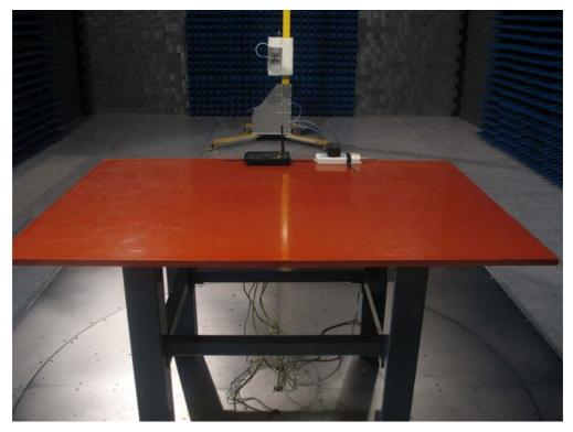
Test Mode: Mode 2: Transmitter by 802.11g Description: Back View of Radiated Test for Above 1GHz
