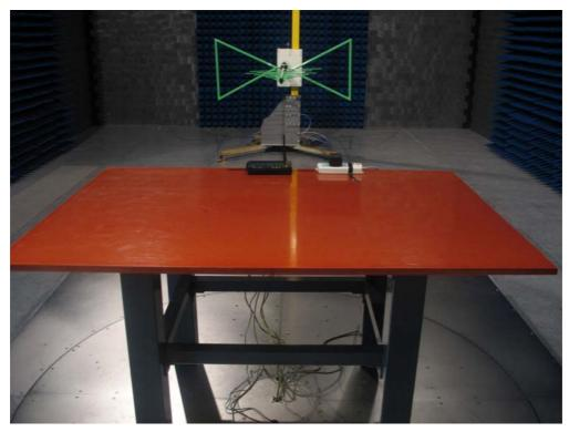
Test Mode: Mode 2: Transmitter by 802.11g Description: Back View of Radiated Test for Under 1GHz
