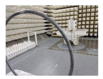
Photograph No.3 Spurious emissions measurement setup in the anechoic chamber in 30 -1000 MHz
