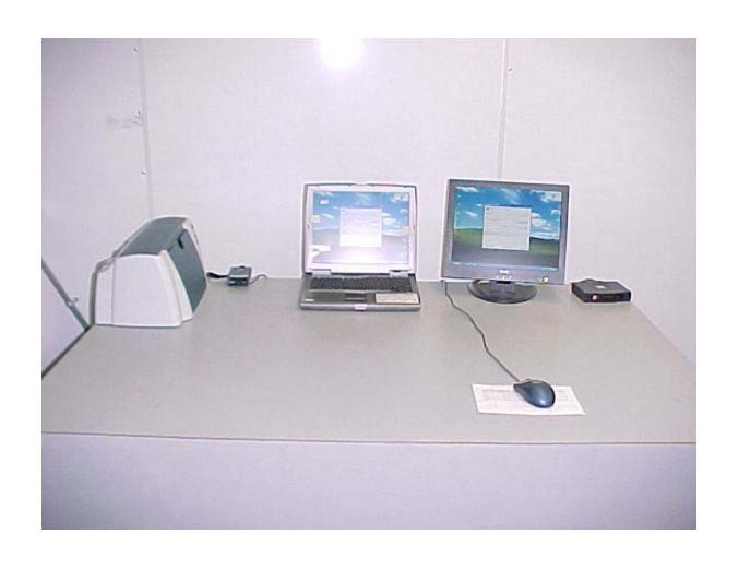
AC Conducted Emissions Measurement (Front View) Setup
