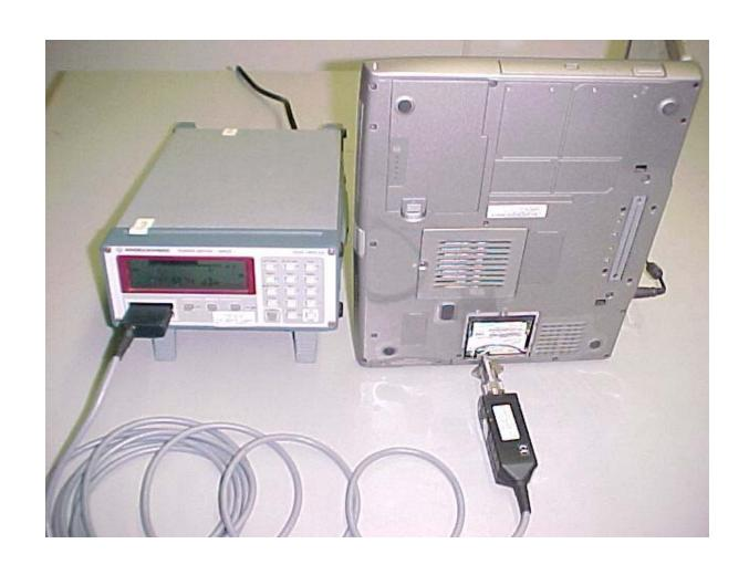
Maximum Peak Output Power Measurement Setup
