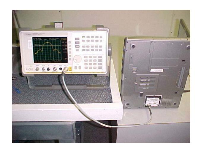
Conducted Emissions at Antenna Terminal Setup
