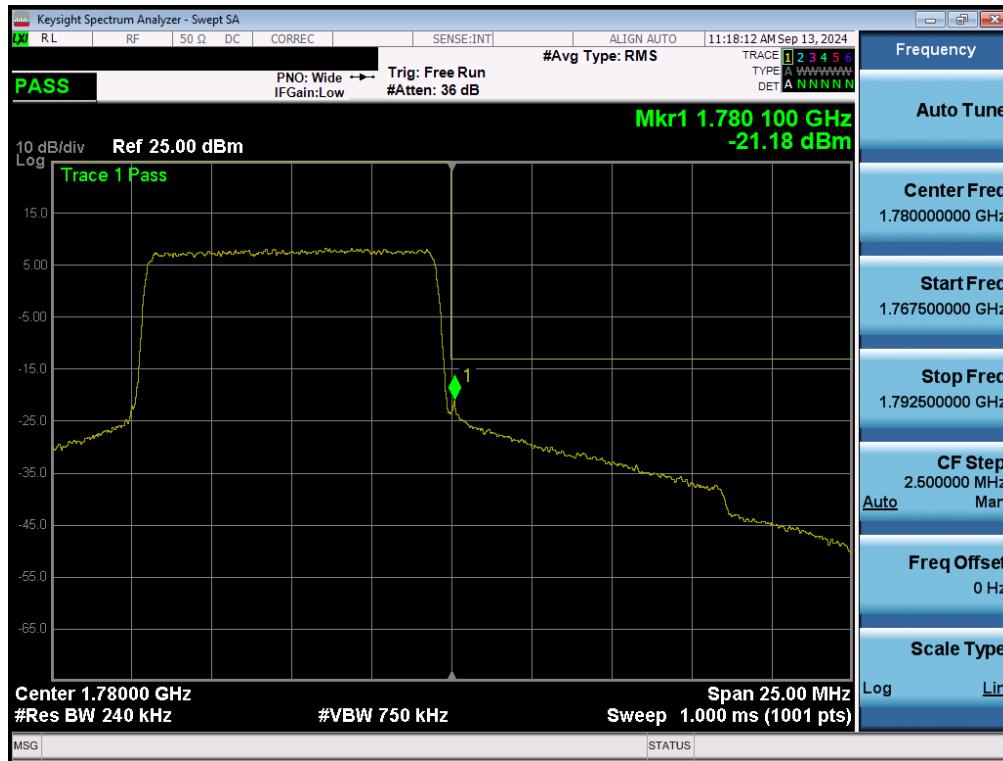
Plot 7-161. Upper Band Edge Plot (LTE Band 66 - 10MHz QPSK - Full RB - ANT2)
