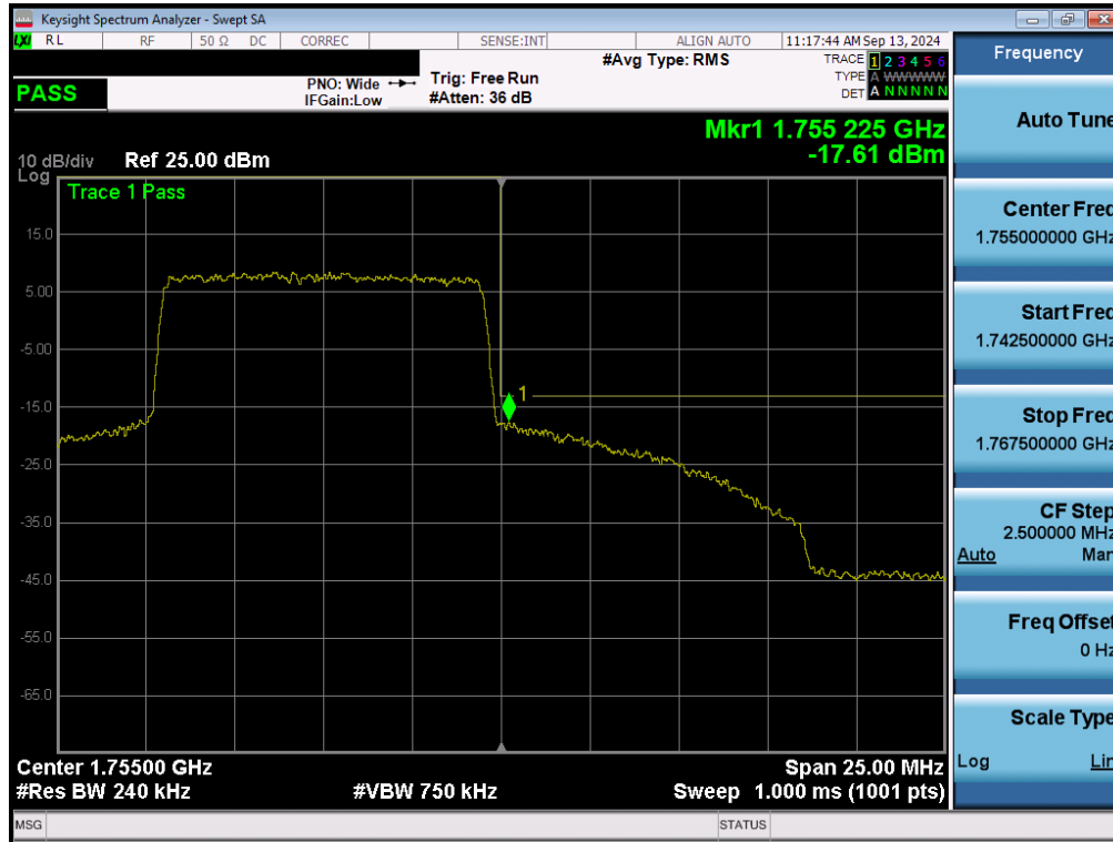
Plot 7-159. Upper Band Edge Plot (LTE Band 4 - 10MHz QPSK – Full RB - ANT2)
