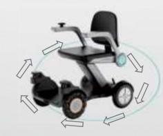
The all-direction wheels offers more stability without being steered 76cm turning radius design for mobility in narrow space
