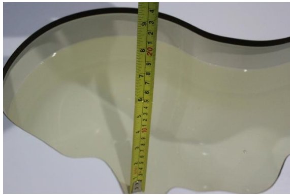
Liquid depth in the head phantom (2600MHz)
