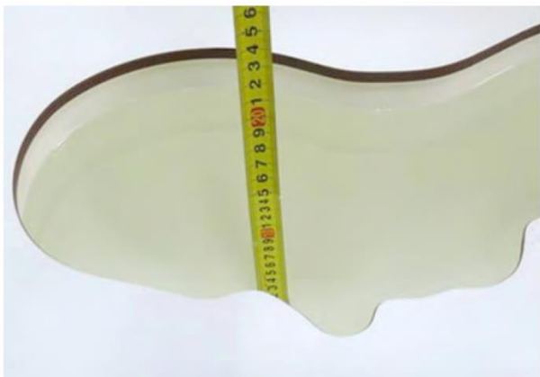
Liquid depth in the head phantom (1900MHz)
