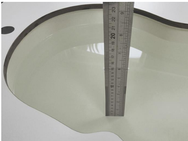
Liquid depth in the head phantom (2450MHz)
