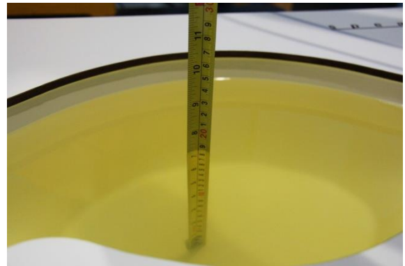
Liquid depth in the body phantom (1750MHz)
