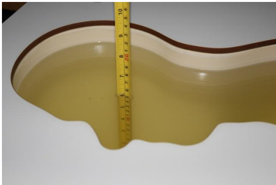
Liquid depth in the head phantom (1750MHz)
