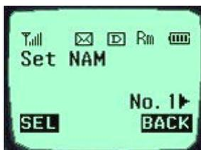
Select one NAM in the two NAM (Number Assignment Module) services. Select either “No. 1” or “No. 2” with the direction key. Both “No.1” and “No. 2” have different NAM parameters, respectively. Therefore, if you select the NAM nidentified with the subscribed number, the service is not available.
