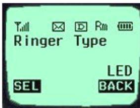
Set one of three ringer types (Ring, Vibrator, and LED) with the direction keys.
