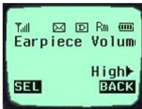
Adjust the earpiece volume in three levels (High > Medium > Low) with the direction keys. It is also adjustable with the side keys in a busy line state.
