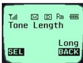
Set the tone length in two levels (Short, Long) with the direction keys.
