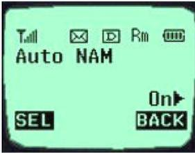
This service enables setting of the NAM to the identified subscribed number for one or more than one NAMs. Use the direction keys to set the service to either “On” or “Off” state.
