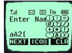
8. Use the Soft Key (CLR) on the right side to erase the input character. Press it for a short period of time to erase the last input character, and press it for some time to erase all the input characters.
