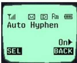
\*\*Note – Press the items in the orders of the Soft Key (MENU) on the left, the [Auto Hyphen] and [ON] items on the screen in a call waiting state to select the Auto Hyphen function.
