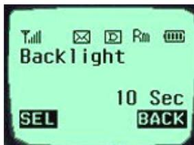
It is possible to adjust the keypad and the backlight time in 5 levels with the direction keys.
