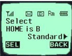
Select either “On” or “Off” with the direction keys. It is possible to select the cellular company with this function.
