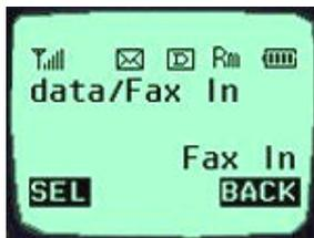
This service enables selection of the data communication type in either the modem termination type or the FAX termination type. Select one of the “Off”, “Data In”, and “FAX In” services, and select the Soft Key (SEL) on the left.
