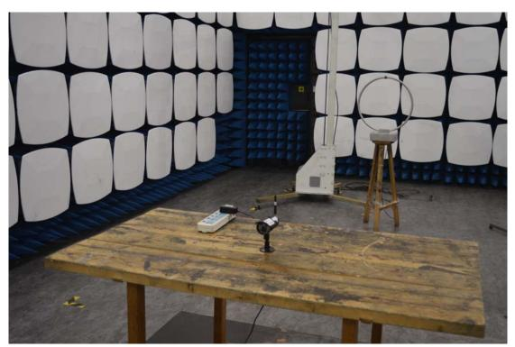
3. Radiated emission (9KHz-30MHz)
