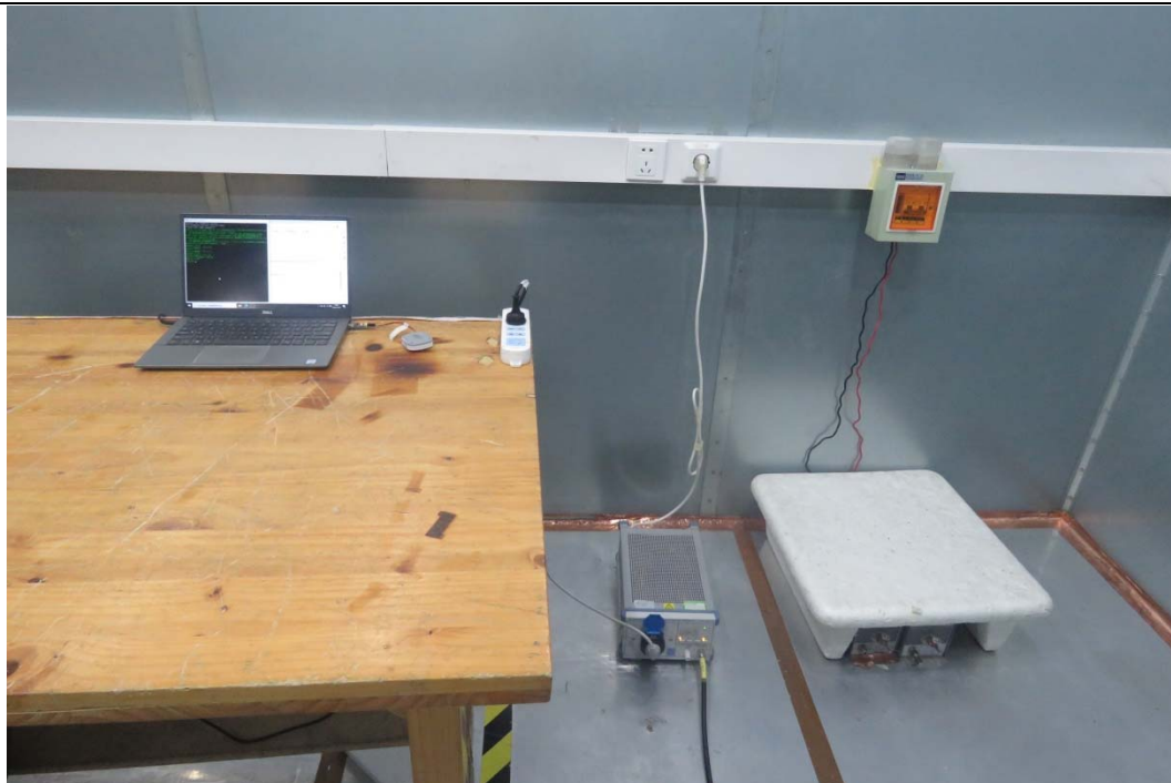
Picture 2 Conducted Emission Test Setup
