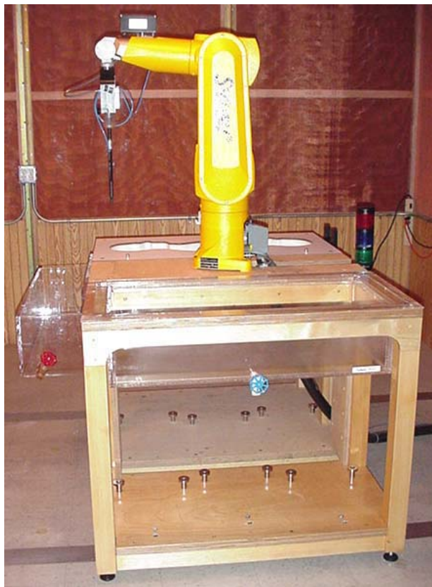
DASY4 SAR Measurement System with validation phantom
