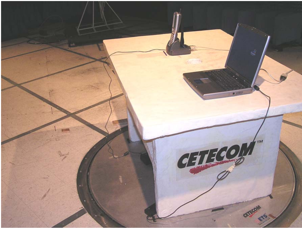
Test setup – Radiated Emissions
