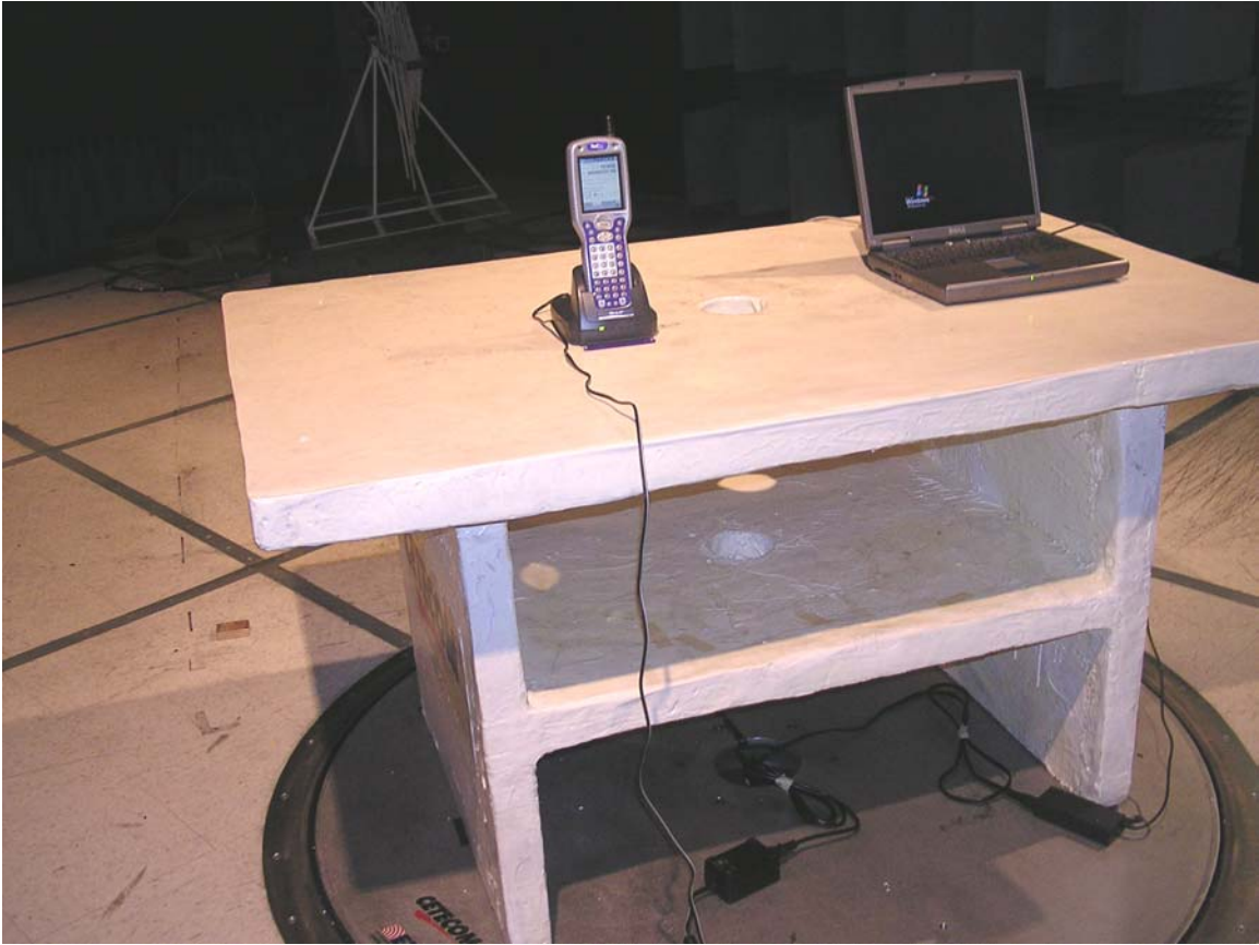
Test setup – Radiated Emissions
