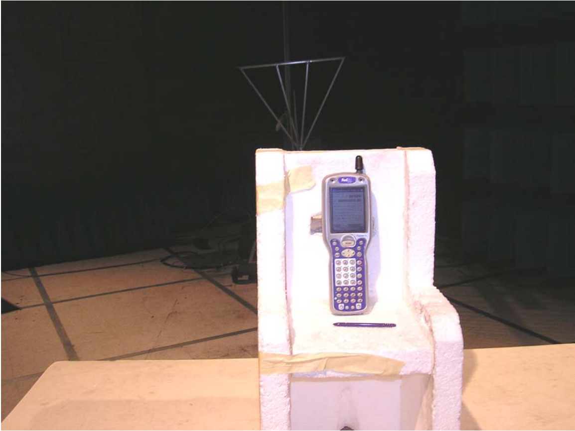
Test setup – Radiated Emissions
