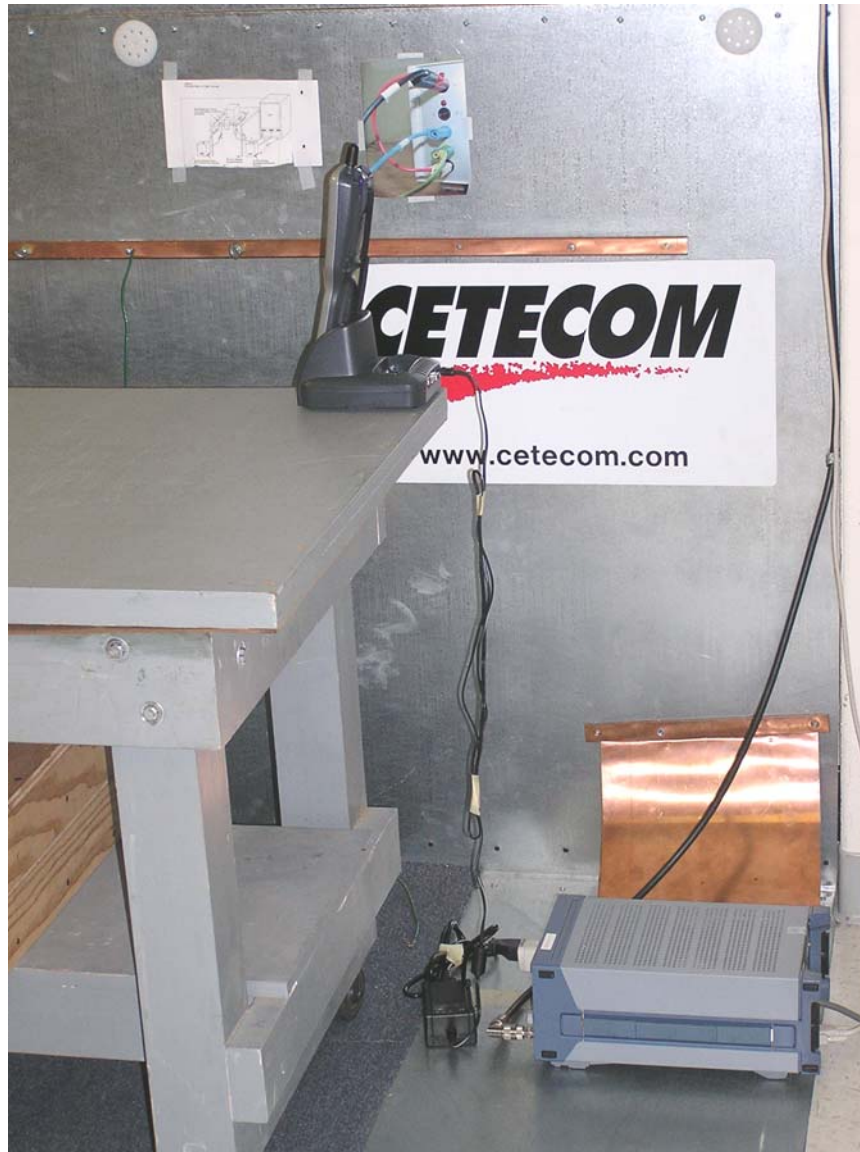
Test setup – AC Line Conducted Emissions
