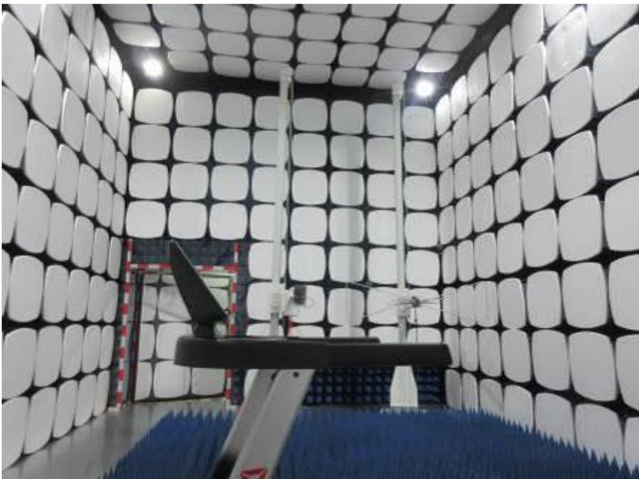
Remark: The transmitter part of the EUT was kept on the high 0.8m below 1 GHz and 1.5m above 1GHz according to the lifting platform during the test.
