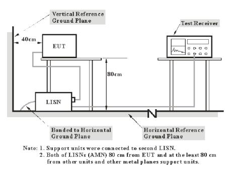
The setup of EUT is according with per ANSI C63.4-2014 measurement procedure. The specification used was with the FCC Part 15 B Class B limits.
