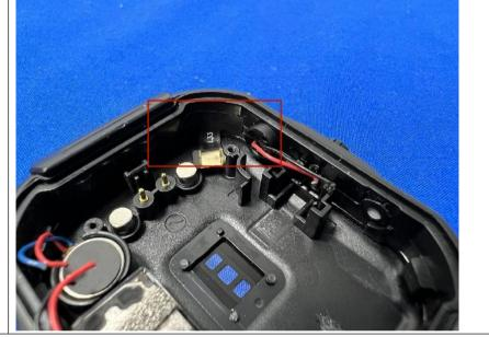
The antenna is FPC antenna. The best case gain of the antenna is -1.23 dBi.
