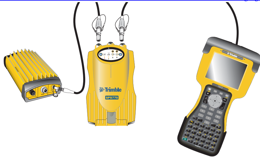
Figure 4.2 Connecting an external radio
