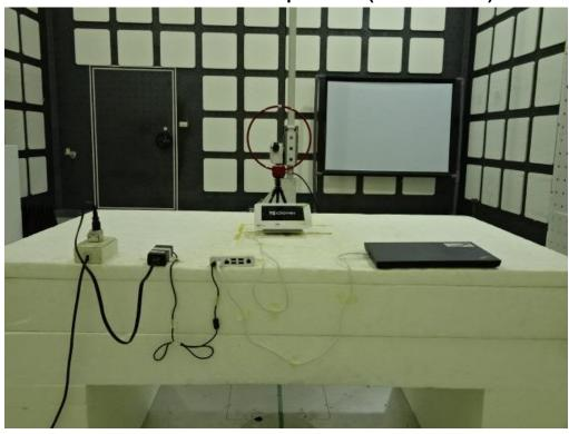
Radiated Emission Set up Photos (Below 1GHz)
