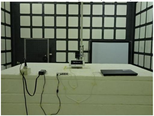
Radiated Emission Set up Photos (Front View)
