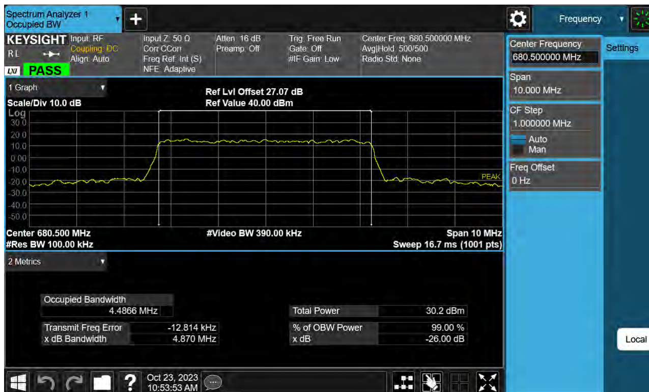
Sub6 n71. Occupied Bandwidth Plot (5 M BW Ch.136100 QPSK_ Full RB)
