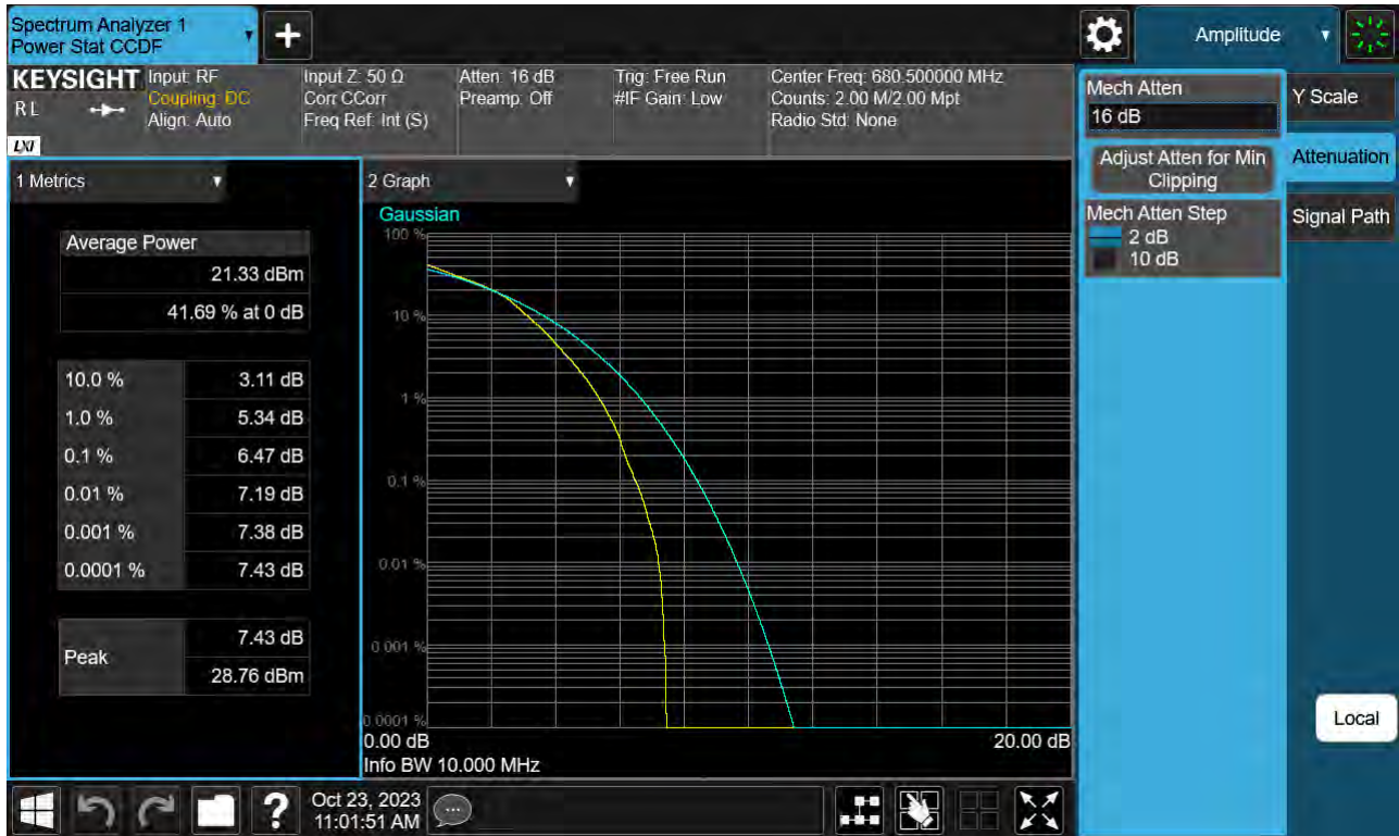
Sub6 n71. PAR Plot (10 M BW_Ch.349000_16QAM_Full RB)
