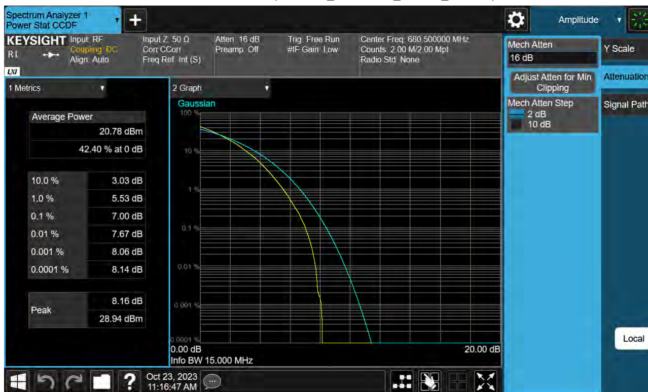
Sub6 n71. PAR Plot (15 M BW_Ch.349000_64QAM_Full RB)
