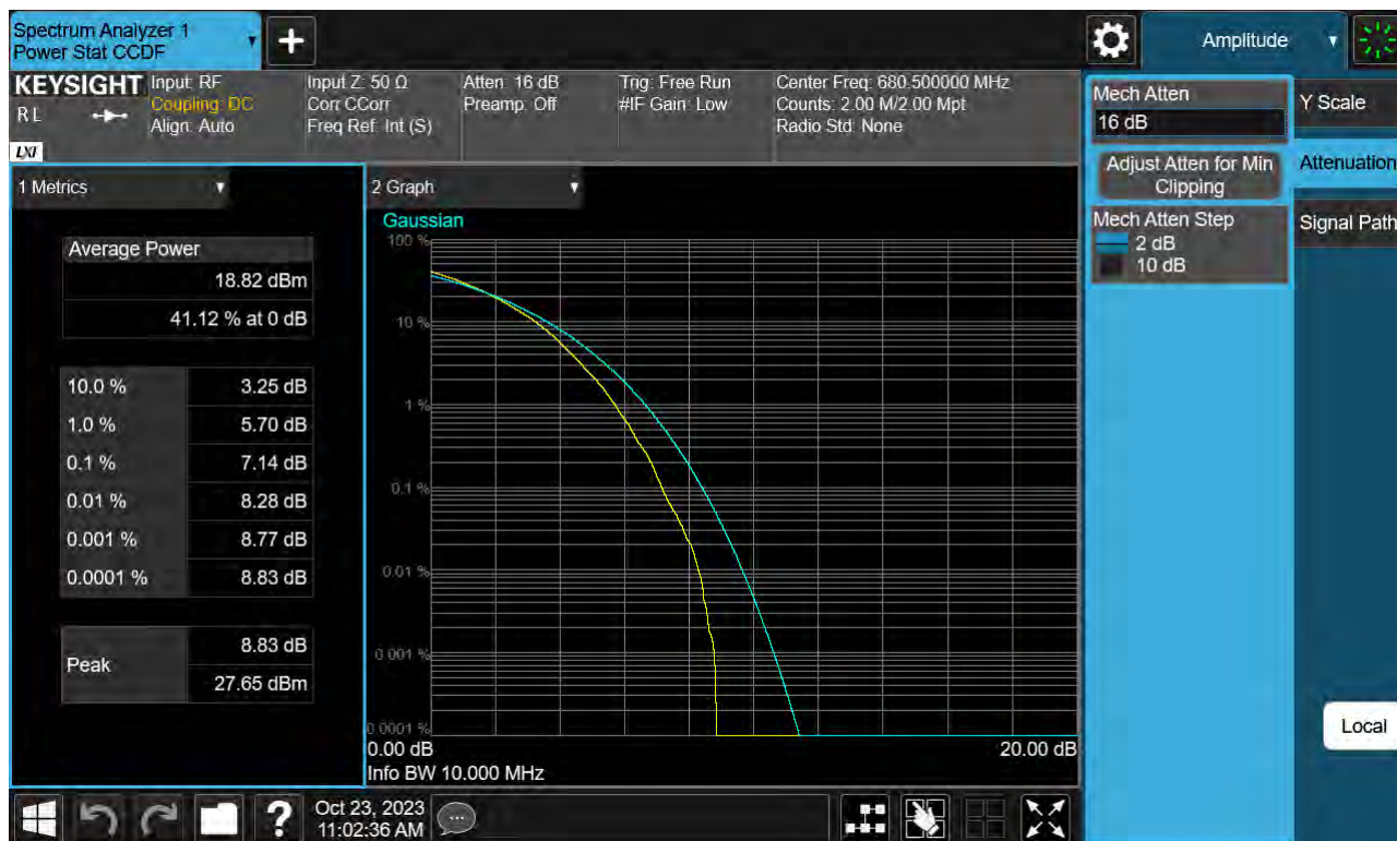
Sub6 n71. PAR Plot (10 M BW_Ch.349000_256QAM_Full RB)
