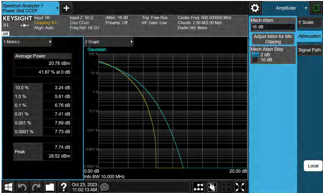
Sub6 n71. PAR Plot (10 M BW_Ch.349000_64QAM_Full RB)
