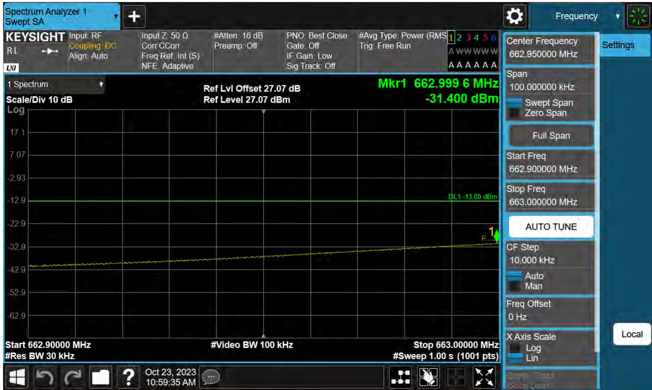
Sub6 n71. Lower Band Edge Plot (10 M BW Ch.133600 BPSK_RB1_Offset 0)_1
