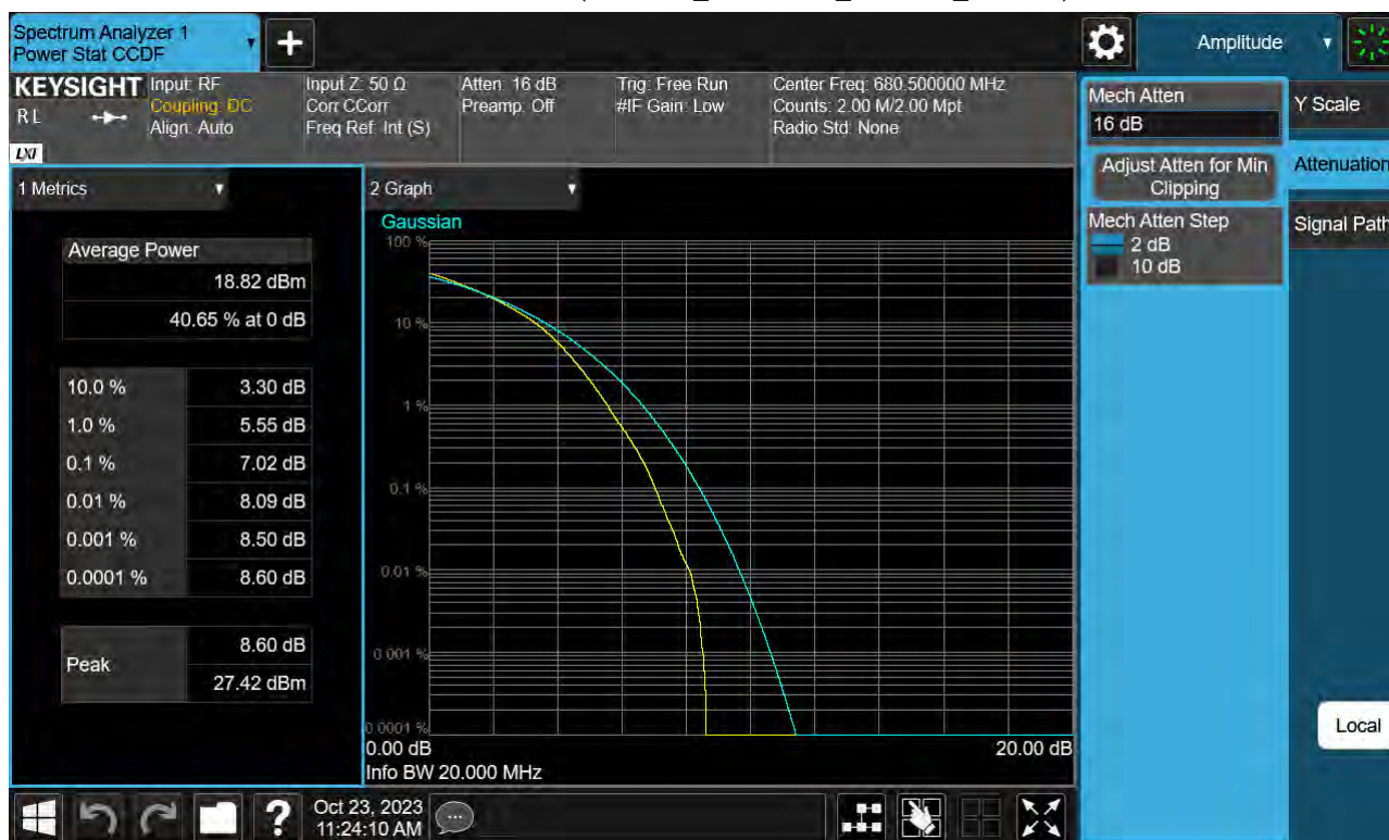
Sub6 n71. PAR Plot (20 M BW_Ch.349000_256QAM_Full RB)
