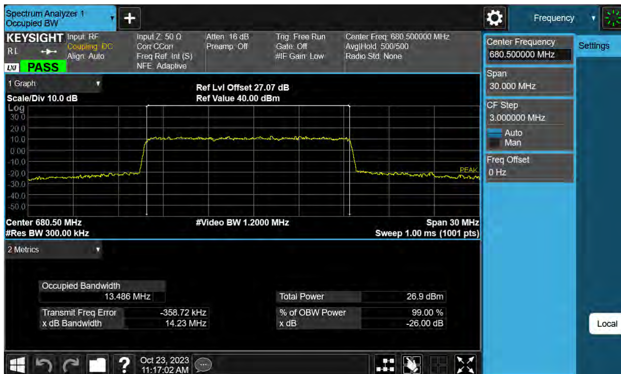
Sub6 n71. Occupied Bandwidth Plot (15 M BW Ch.136100 256QAM_ Full RB)
