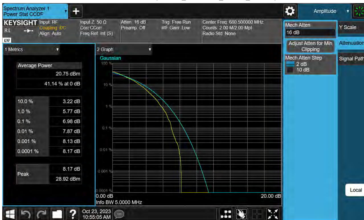
Sub6 n71. PAR Plot (5 M BW_Ch.349000_64QAM_Full RB)
