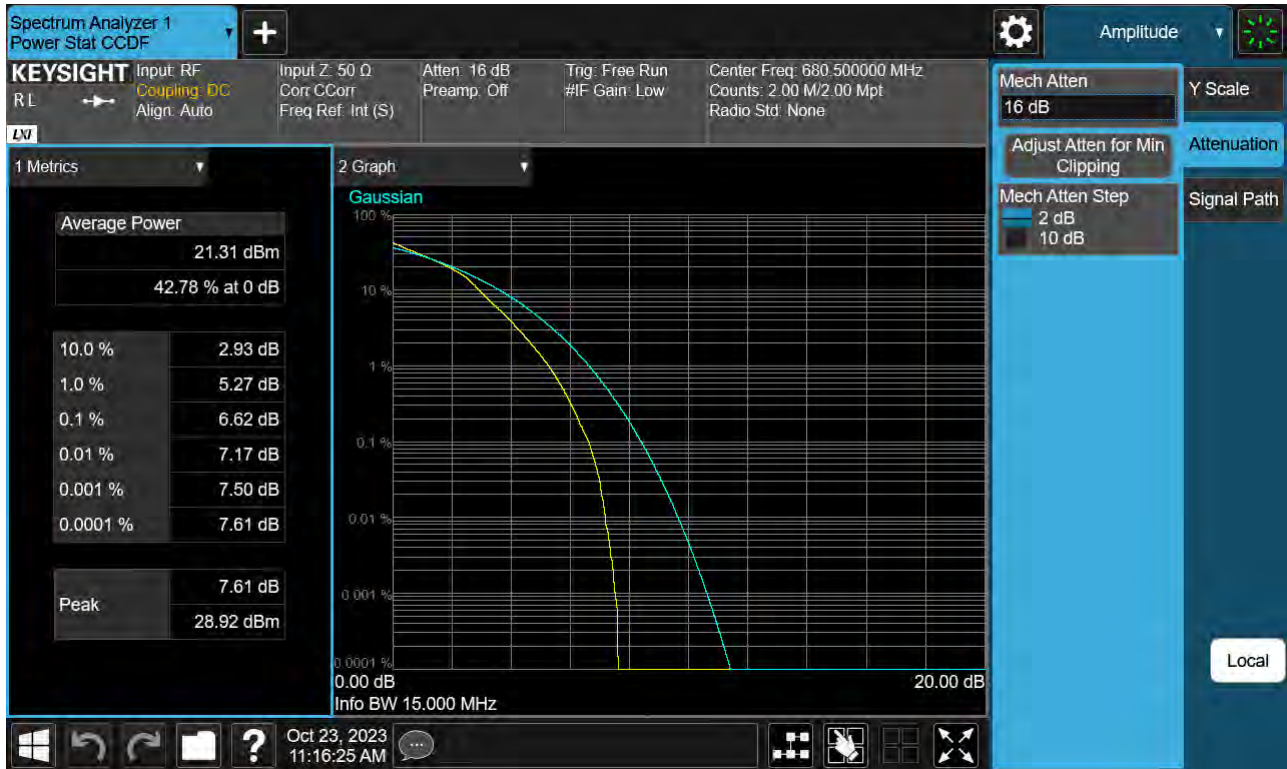
Sub6 n71. PAR Plot (15 M BW_Ch.349000_16QAM_Full RB)
