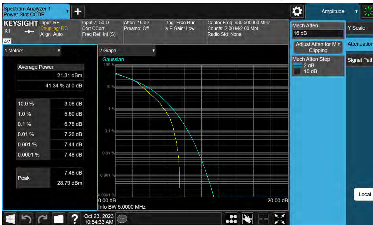
Sub6 n71. PAR Plot (5 M BW_Ch.349000_16QAM_Full RB)
