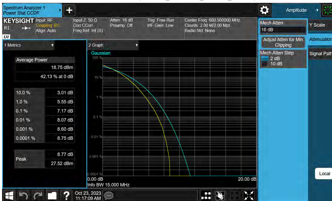
Sub6 n71. PAR Plot (15 M BW_Ch.349000_256QAM_Full RB)
