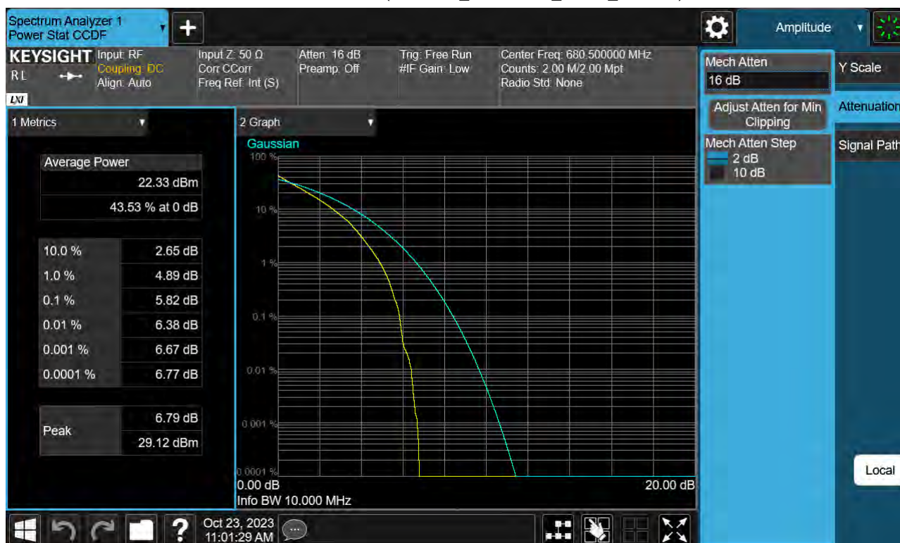
Sub6 n71. PAR Plot (10 M BW_Ch.349000_QPSK_Full RB)
