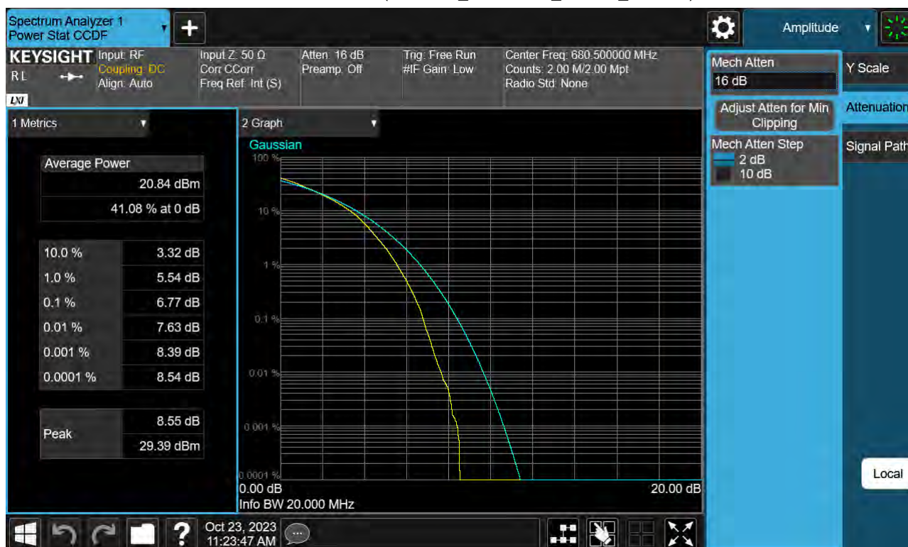
Sub6 n71. PAR Plot (20 M BW_Ch.349000_64QAM_Full RB)
