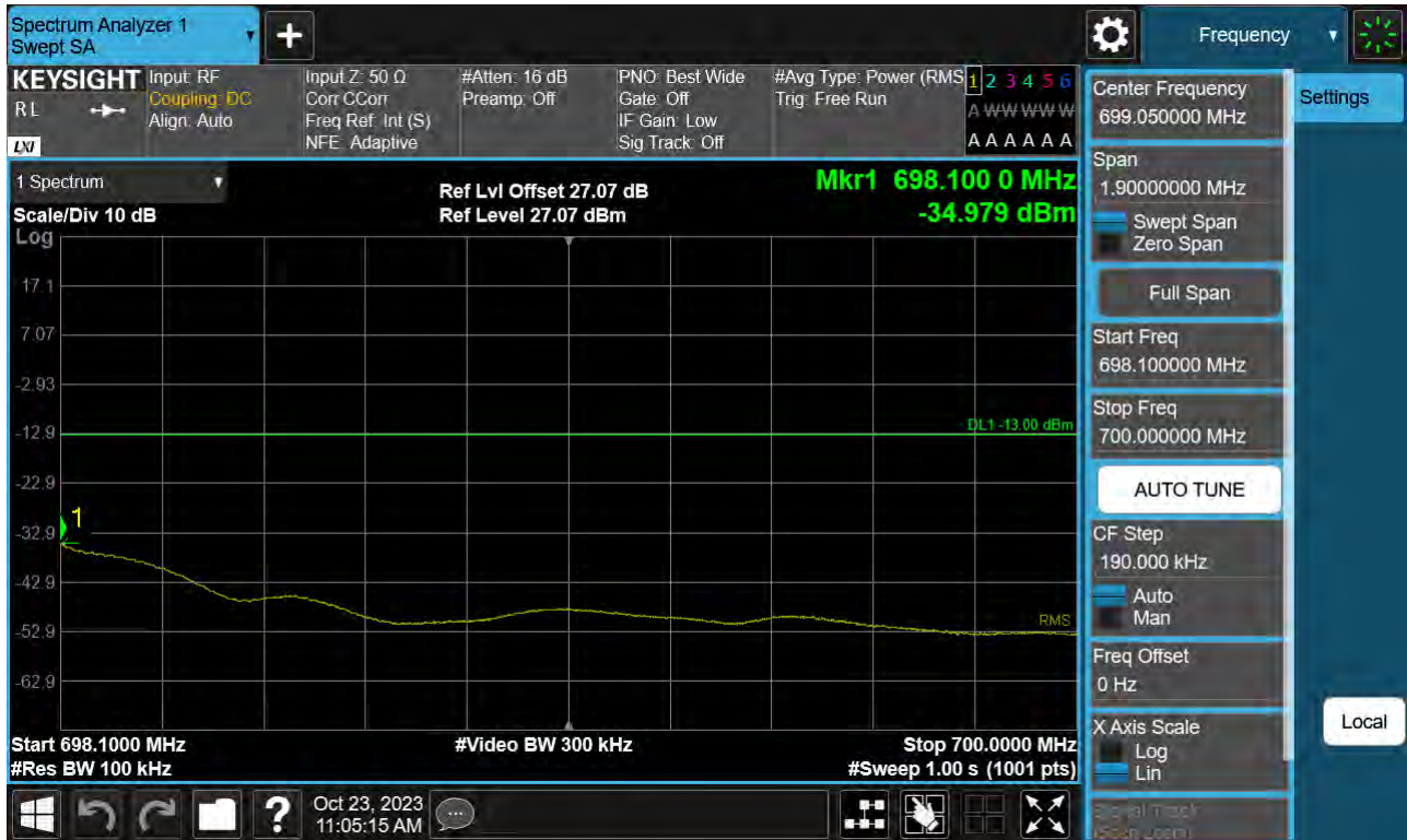
Sub6 n71. Upper Band Edge Plot (10 M BW Ch.138600 BPSK_RB1_Offset 51)-2
