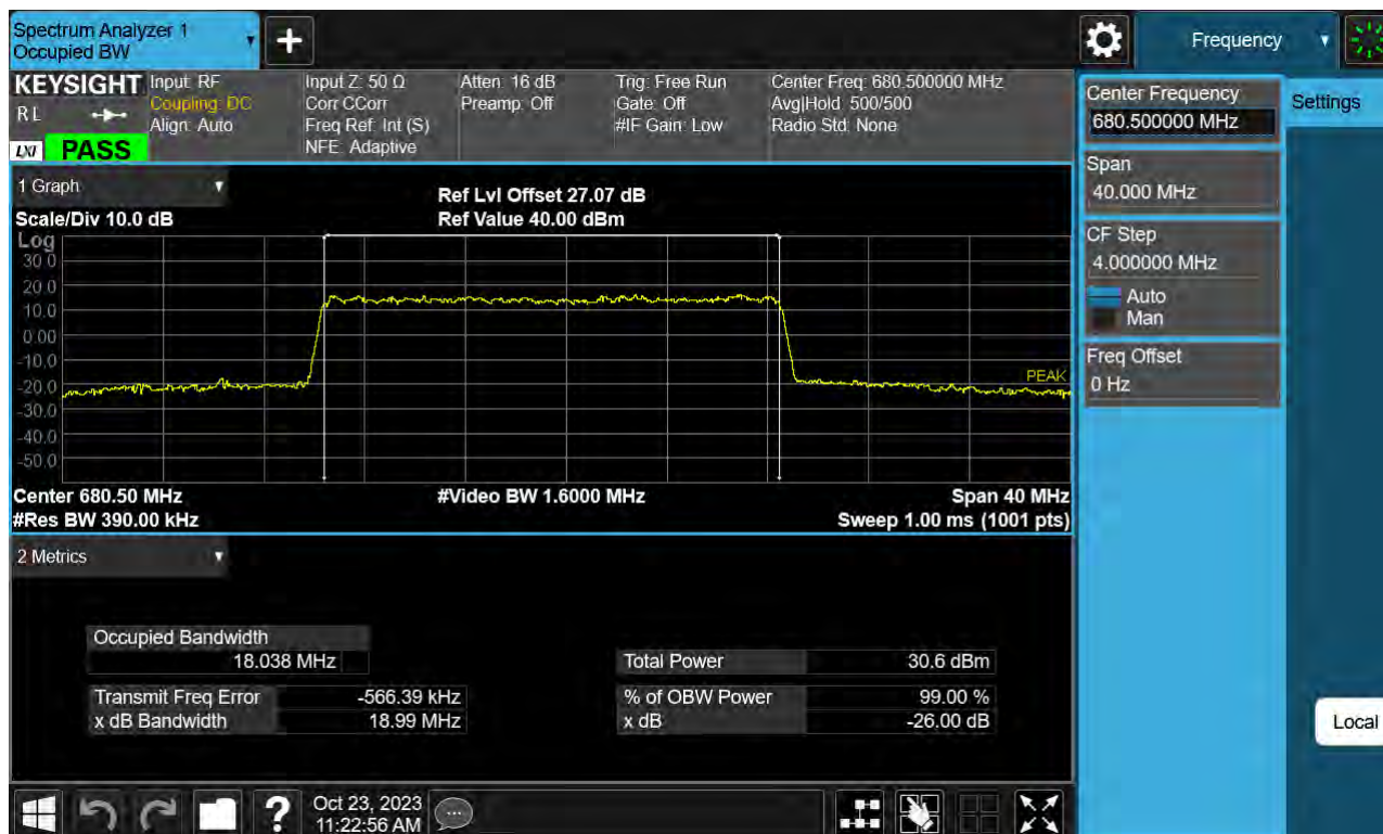
Sub6 n71. Occupied Bandwidth Plot (20 M BW Ch.136100 QPSK_ Full RB)
