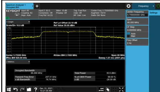
802.11ac-VHT80 26dB &amp; 99% Bandwidth
