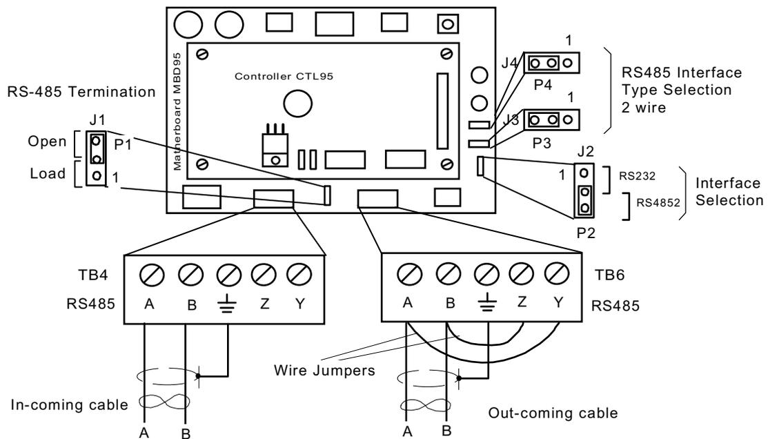
Figure 2-2: Connections and Jumper Settings for the RS-485 Two-Wire Communication Line
