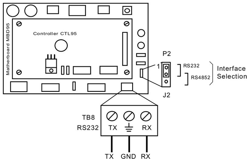
Figure 2-1: Connections and Jumper Settings for the RS-232 - PC Communication Line
