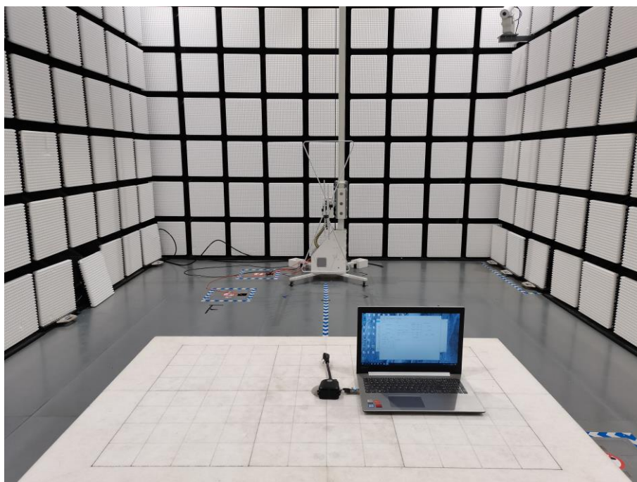
Fig. 2 Radiated emission setup photo(30MHz-1GHz)
