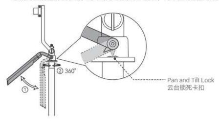
Loosen the knob to adjust the angle up and down. Tighten the knob after completing the angle adjustment,
