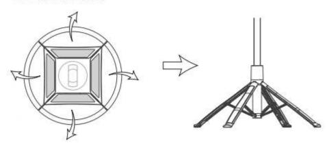
Hold the sleeve and pull it down to the bottom to extend the legs to their maximum angle. Then, place it on a flat surface.
