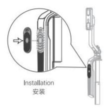
Shutter button: Short press for 1 second to take photos and record videos, long press for 3 seconds to power on/off. The indicator light will flash quickly 3 times when powering on/off.
