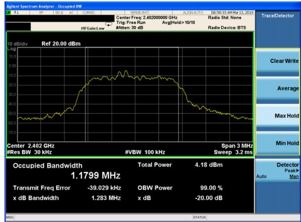
20dB Bandwidth plot on channel 39 (1Mbps)
