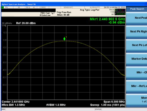
Peak output Power plot on channel 78 (3Mbps)
