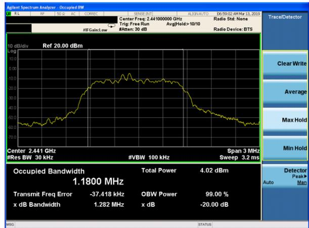
20dB Bandwidth plot on channel 78 (1Mbps)
