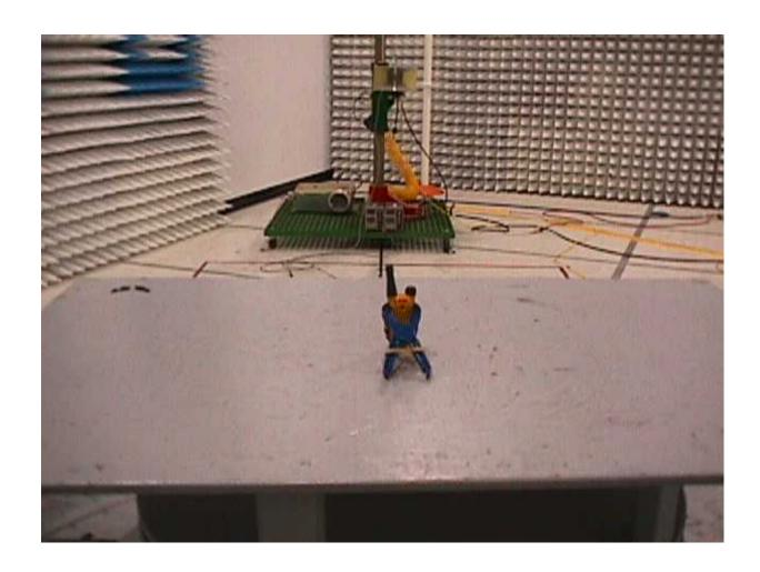
**Radiated Emissions Test Configuration**
