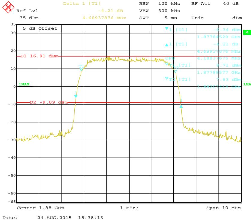
**99% Occupied & 26 dB Emissions Bandwidth for HSDPA (16QAM) Mode**
