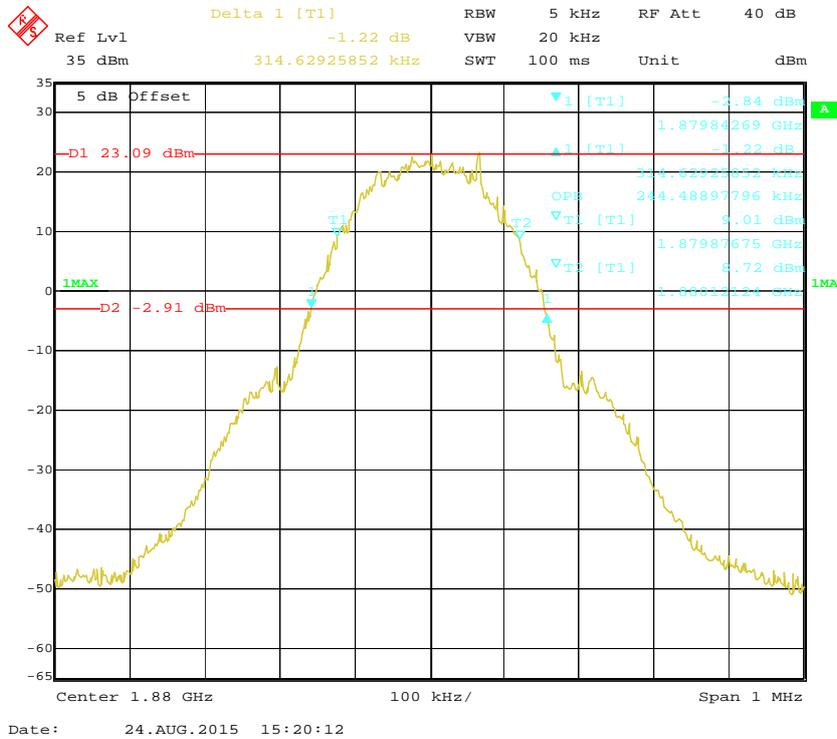
**99% Occupied & 26 dB Emissions Bandwidth for EGPRS (8PSK) Mode**
