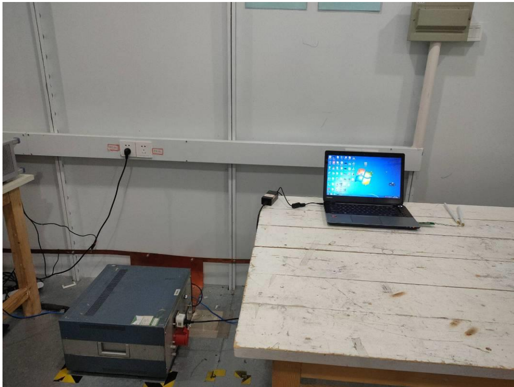
Photo of Conducted Emissions Measurement
