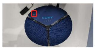
e) After the boot is completed, press the live key, one of the top indicatie lights will start flashing and the upgrade will start.
