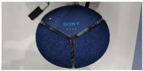
g) Then the third and fourth lights flashed blue. the machine restarts automatically and the upgrade is successful
