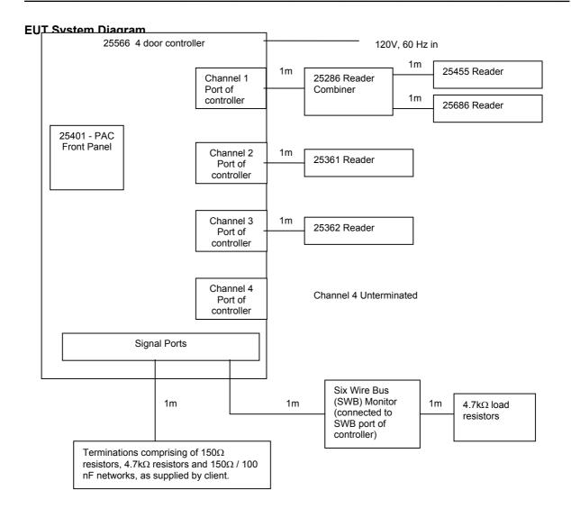
NOTE: The controller is support equipment (it is not being tested). It is submitted only to allow us to perform the Conducted and Radiated emissions tests on the other units.
