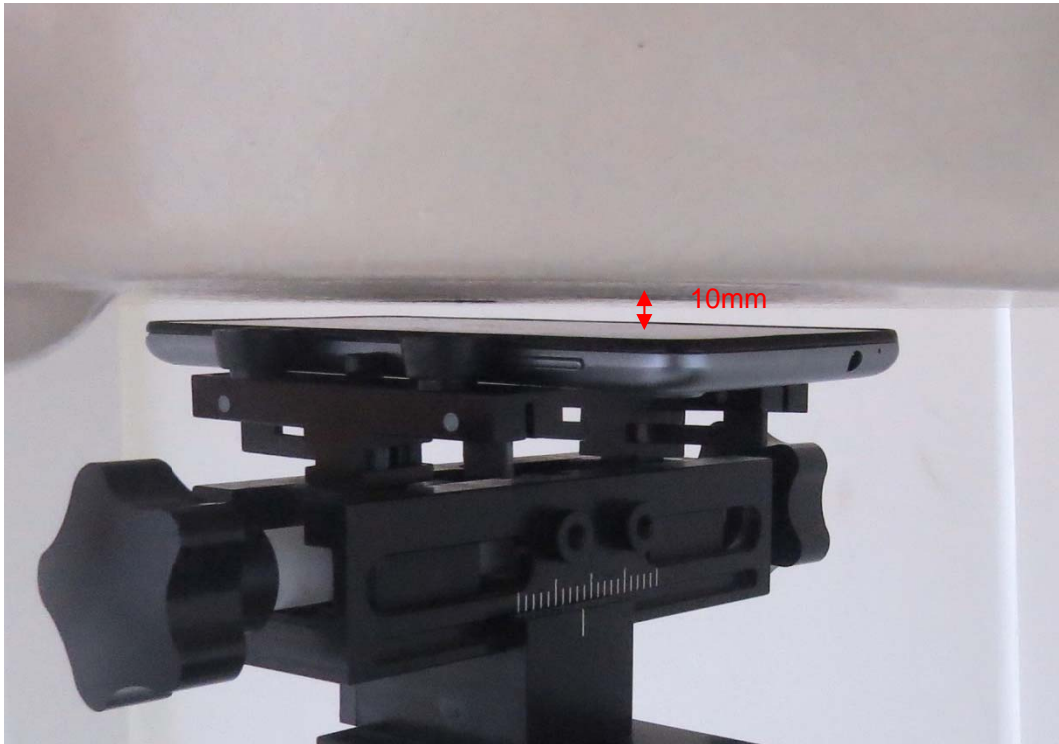
Picture 9: Front Side, the distance from handset to the bottom of the Phantom is 10mm
