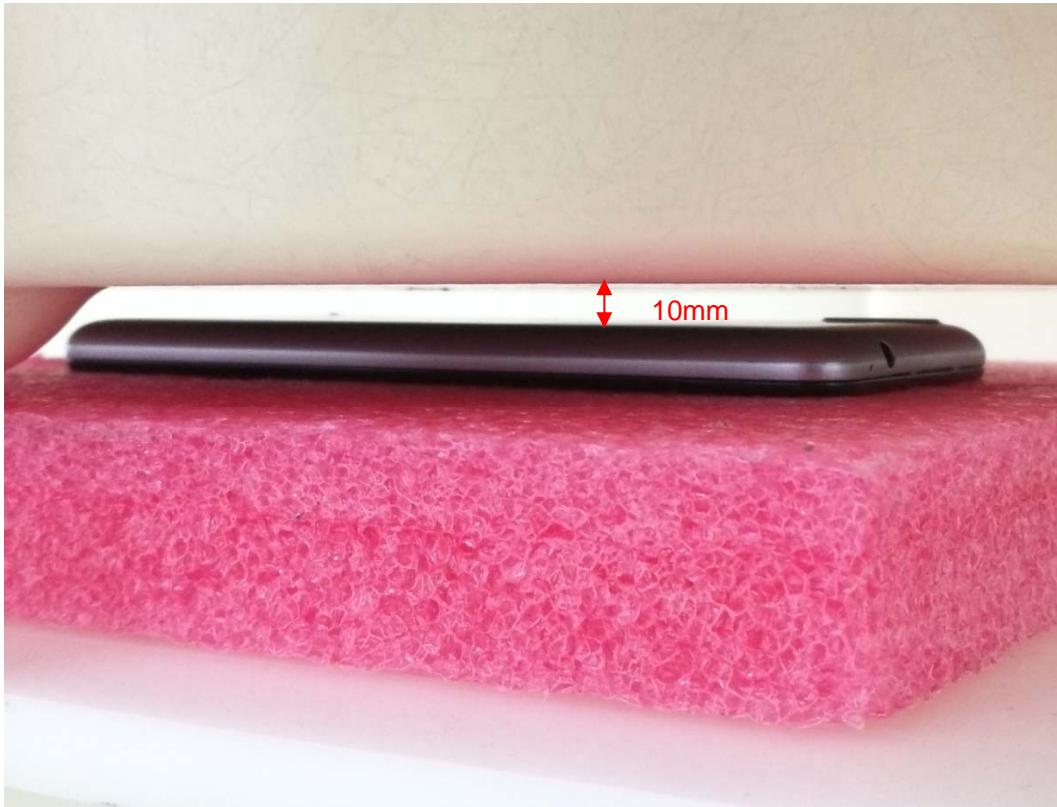
Picture 7: Back Side without holder, the distance from handset to the bottom of the Phantom is 10mm
