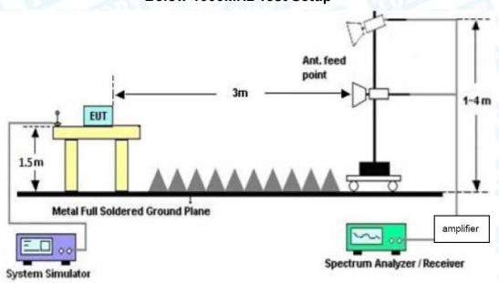
**Above 1GHz Test Setup**
