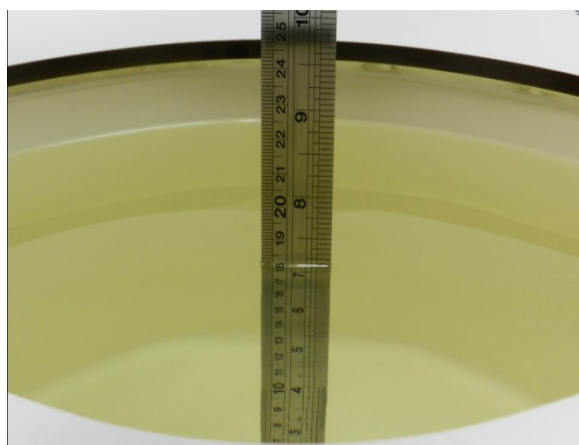
Fig 10.2 Photo of Liquid Height for Body SAR
