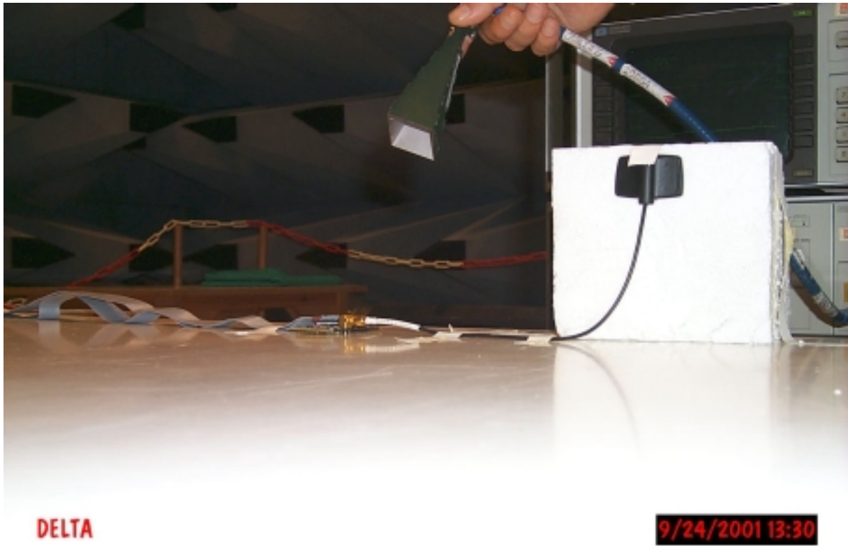
PHOTO A2.5 Test set-up for test 18-26 GHz
