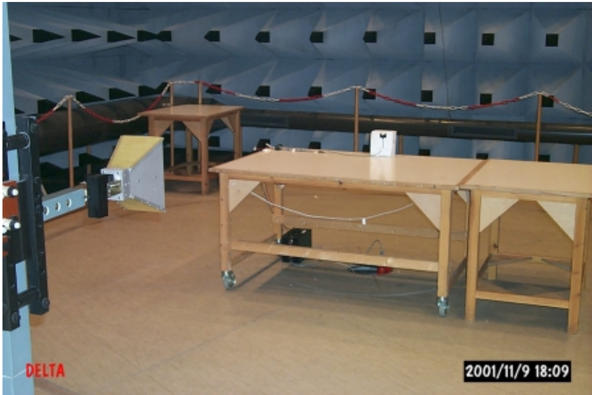
PHOTO A2.3 Test set-up for test 1-12.75 GHz
