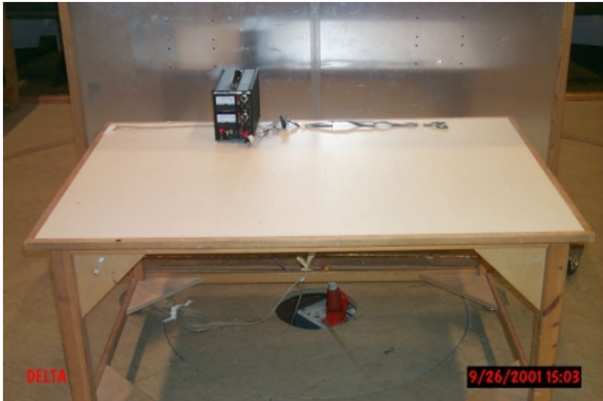
PHOTO A2.1 Conducted emission
