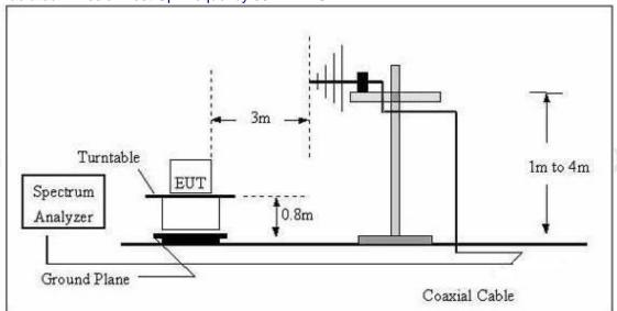
(C) Radiated Emission Test-Up Frequency Above 1GHz
