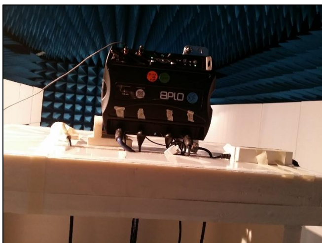
Configuration n°3 Test setup in anechoic chamber >1GHz
