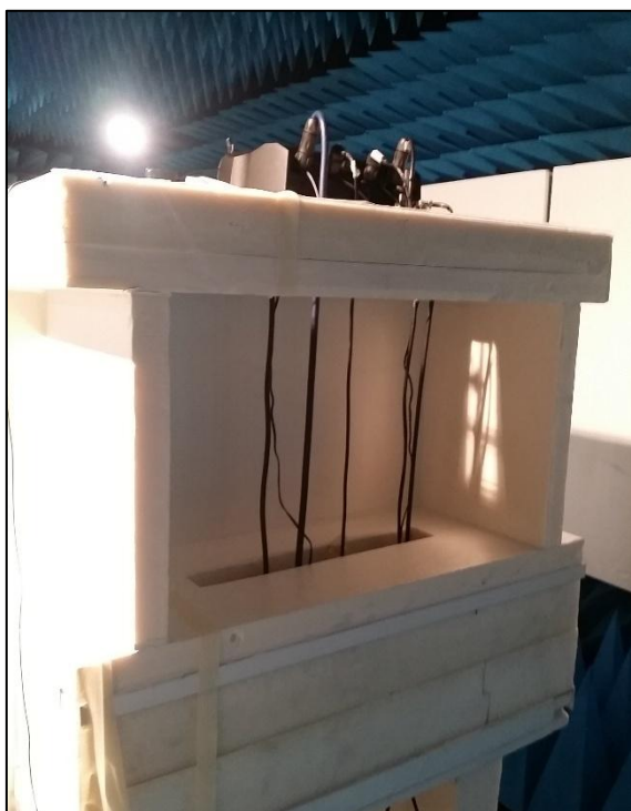
Configuration n°2 Test setup in anechoic chamber >1GHz
