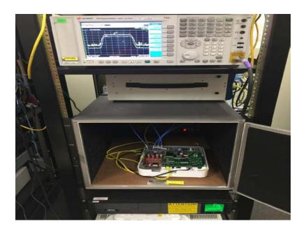
Radiated Test Setup 1-40GHz
