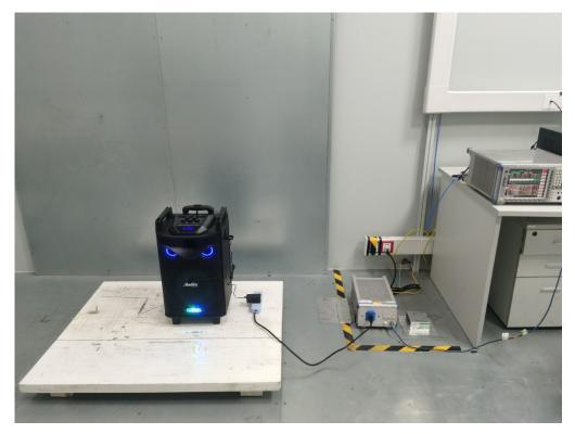
Radiated emission test 30MHz – 1GHz
