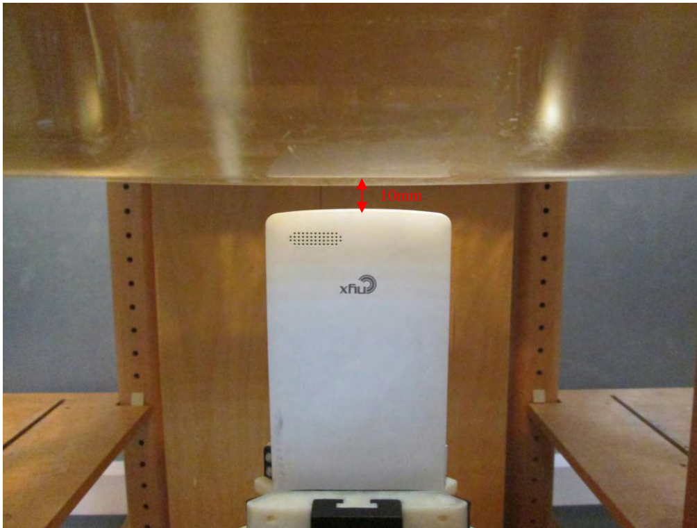
Body-worn Bottom Setup Photo (10mm)
