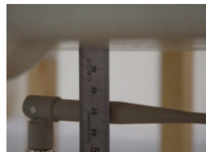
Fig. 21. Body SAR Test Setup with Holster
