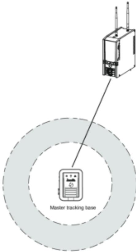
Check first the status of the **Power supply indicator** of the Master tracking base. This LED lights up in green and remains steady when the power supply is correctly provided. Check then the physical communication between the Master tracking base and CONNECT.
