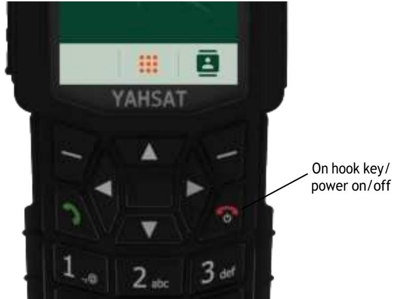
If the handset does not start up, the reason may be that there is no PoE in the LAN interface. If you are connecting to a satellite terminal, check that you are connecting to the right LAN interface with PoE, and that PoE is enabled in the satellite terminal. For further information, refer to the manual for the satellite terminal.
