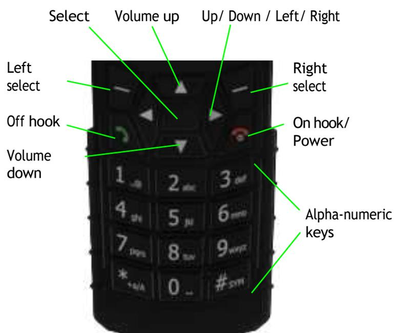
The next sections explain the functions of each key in the keypad.
