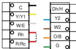
Combined Single Stage Heat and Single Stage Cool with C-Wire Furnace and Air Conditioner.
