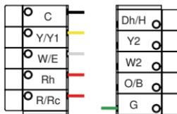
Single Stage Heat/Two Stage Heat Pump with Emergency Heat and Auxiliary Heat with C-Wire.
