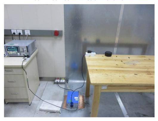
FCC RADIATED EMISSION TEST SETUP
